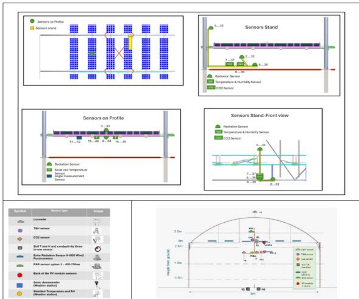
Figure 18. Position and type of the different sensors inside the greenhouses in all locations.
