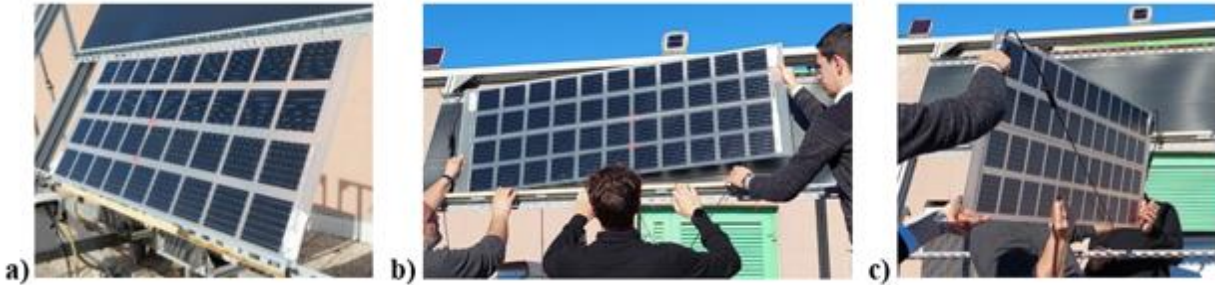
Figure 1. Execution of phase 1 – PV panel acceptance: a) I-V curves for the full functionality test are acquired; b) the panel's rear side is covered for the front functionality test; c) the module is flipped for the rear functionality test.
