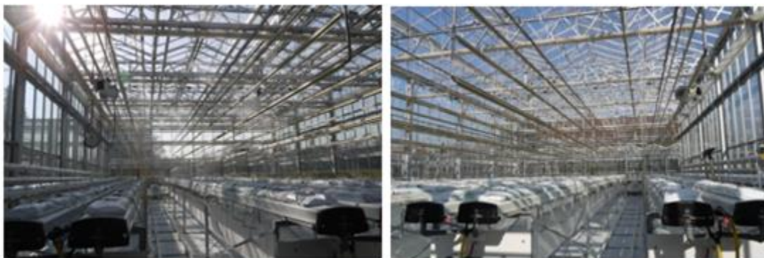
Figure 164. Experimental greenhouses at Humboldt University in Berlin; on the left, the collector greenhouse with technical cooling and maximum thermal insulation before the installation of PV elements; on the right, an identical reference greenhouse with conventional equipment.
