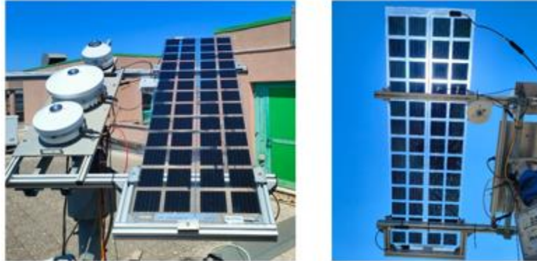
Figure 8. Front and rear view of the experimental setup for the measurement of BiFi.
