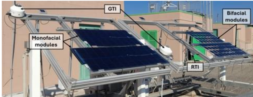
Figure 11. Experimental setup for performance and degradation testing.
