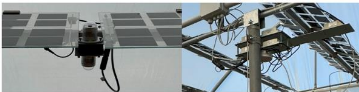
Figure 43. PV monitoring sensors: GTI & RTI (left), luxmeter, Temperature & relative humidity, CO 2 and TBOM sensors (right).
