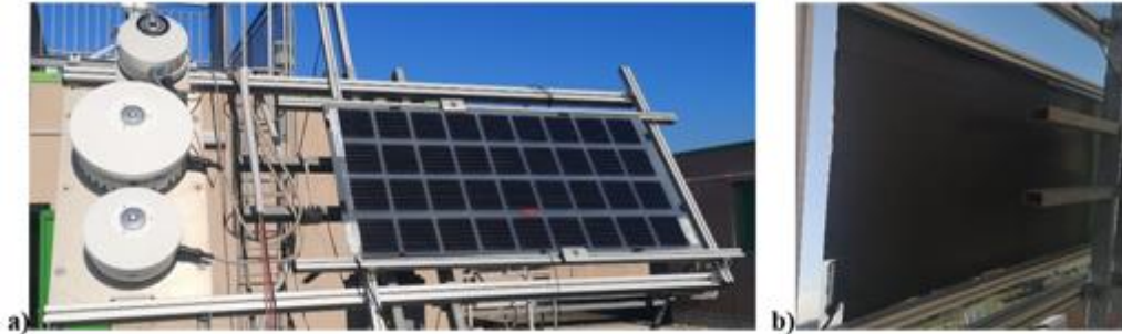
Figure 4. Experimental setup for the measurement of temperature coefficients: a) module positioned on the tracker stand, b) rear side covered by the black sheet.
