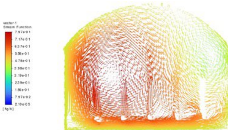
Fig. D.69 Streamlines for 14/05/24 with cucumber plants, without PV panels at 12.00 [h]
