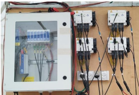
Fig. 6: PV I-V measurement system, including I-V measurement blocks, irradiance block and module temperature block
