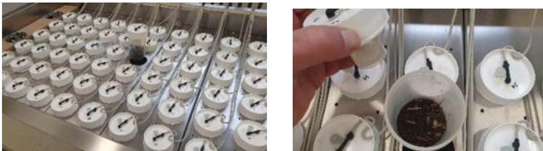
Figure 7 Unit for measuring CO 2 -emission; transfer mulch sample for CO 2 absorption
