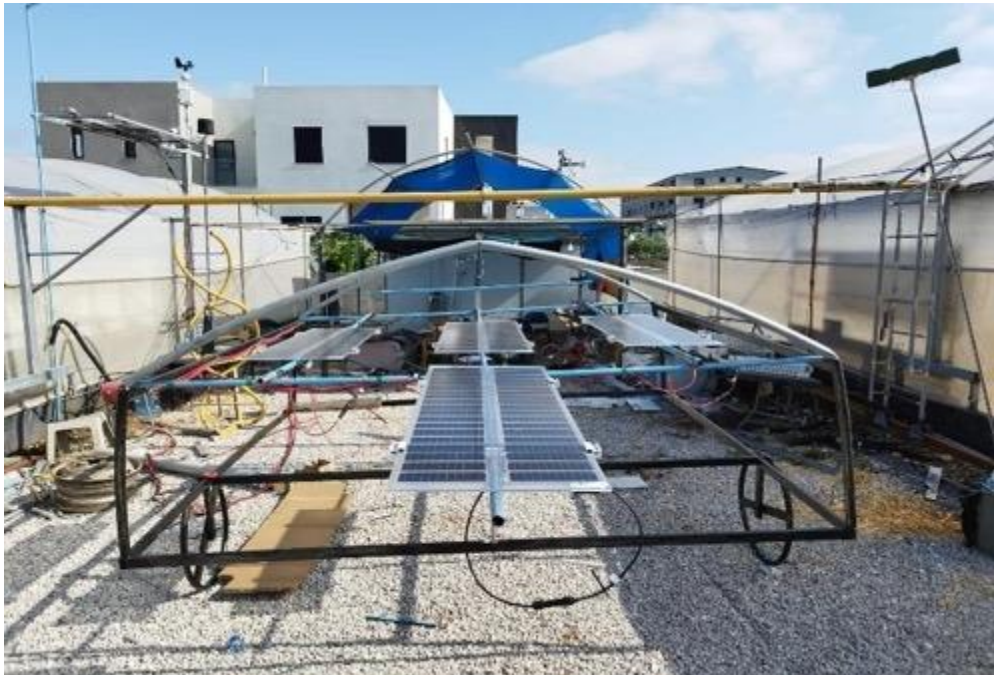
Figure 9 PV modules sample testing
